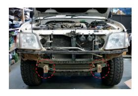
3. Fit chassis bracket to chassis using M10 bolts, flat washers and spring washers into original bumper bolt holes. Refit original recovery hook on right hand side and tie down point on left hand side using original bolts.
